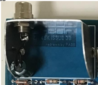
tin-plated copper sheet for mounting the socket
